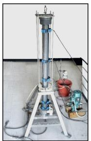
Figure 1: Laboratory equipment for penetrability evaluation [9-15].
