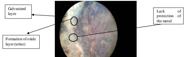
Figure (4): Surface of the part of an element of angular profile in structure of the Najasa model.
