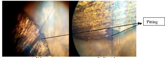
(a) Urban (b) Coastal Figure (3): Cross section of circular profile elements in structures AT-60 model
