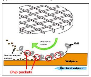
Figure 6: Wafer saw mechanism showing how chipping pockets occur
