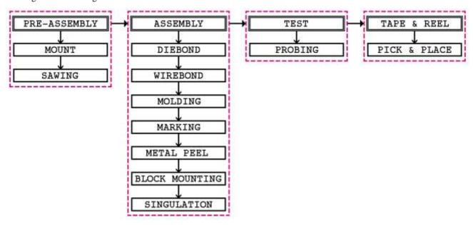
Figure 3: Device A complete process flow
