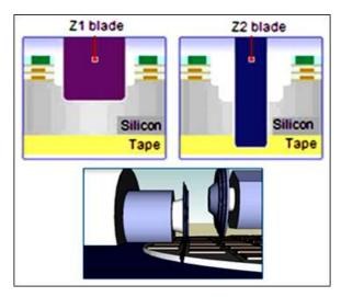
Figure 9: Step-cutting method
