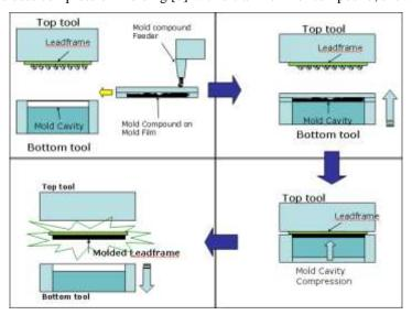
Figure 10: Compression molding mechanism
