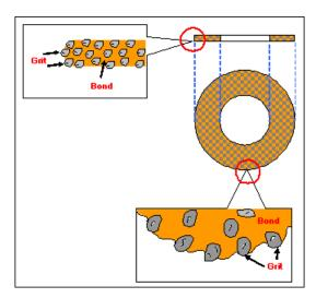
Figure 7: Elements of blade structure and their purpose
