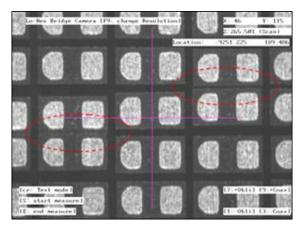
Figure 11: Singulated units showing narrow gaps in between units, resulting to auto align (AA) failures
