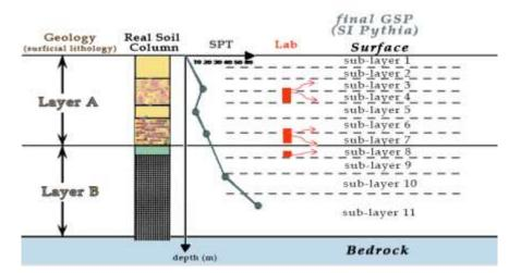
Figure 4: An Example on How a Geotechnical Soil Profile (GSP) is Created by SI
