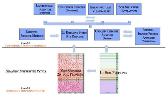
Figure 1: SI (Level 3) Establishes Geotechnical Semantics to Increase the Productivity of *GeoSeism* and the Related Interoperable GIS (Level 4) [Source: [3]]
