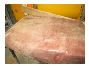
Figure 1: Sample in curing pouch
