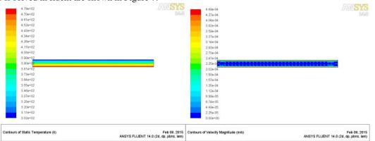
Figure 7: Temperature and velocity contour of Horizontal Plate
