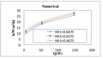
Figure 11: Heat Transfer Coefficient Vs Power by Numerical
