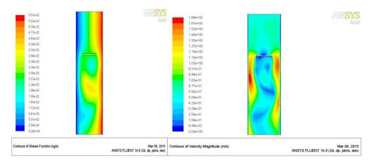
Figure 12: Stream line and Velocity Contours of horizontal plate in vertical channel.
