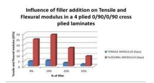
Figure 6 Filler influence on Tensile and Flexural modulus in 4 plied laminate
