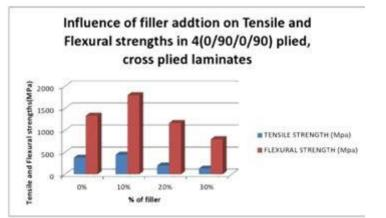
Figure 5 Influence of filler on Tensile and Flexural strength in 4 plied laminate
