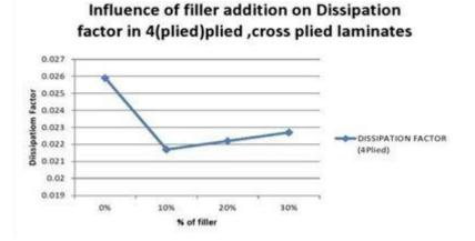
Figure 9 Filler influence on Dissipation Factor in 4 plied laminates Table 2. Mechanical properties
