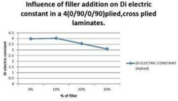
Figure 8 Filler influence on Di electric Constant in 4 plied laminate
