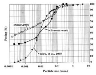
Figure 4: Grain size distribution diagram for sample (L.P.C.C) compared with previous studies.
