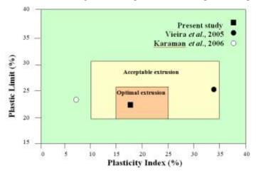
Figure 5: Natural sample (L.P.C.C) optimization according to Atterberge limits comparing with previous studies.
