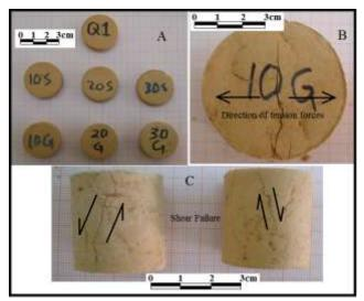
**Figure 2:** Three types of prepared samples for engineering tests, A: small disc has diameter 30.6 mm., B: large disc has diameter 63.6 mm. and D: cylinder has diameter 30.6 mm., Q1 is the natural clay material (L.P.C.C) without any additives, the numbers 10-30 means the percent of additives of sand S or glass G, note photos B and C after test.
