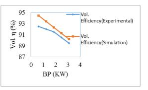
Figure6: Variation of Volumetric Efficiency w.r.t BP
