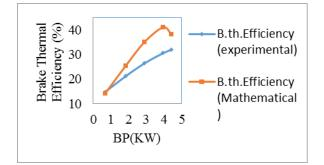
Figure9: Variation of Brake Thermal Efficiency w.r.t Load
