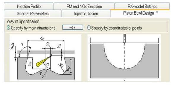
Figure1: Hemispherical Piston Bowl Modelled with Diesel
