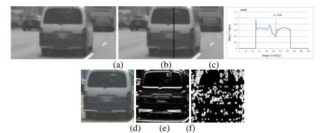
Figure 10: The vehicle verification for a hit case: (a) median filtering result of vehicle candidate image, (b) (c) symmetry measurement result, (d) vehicle candidate region, (e) horizontal edge detection result, (f) vertical edge detection result.
