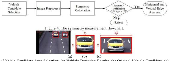
Figure 5: Vehicle Candidate Area Selection: (a) Vehicle Detection Results, (b) Original Vehicle Candidate, (c) Vehicle Candidate Symmetry Measurement Area.
