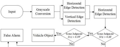
Figure 7: The horizontal and vertical edge analysis flowchart.
