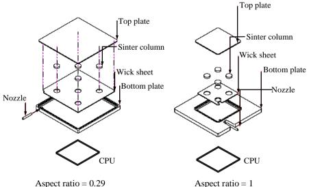
**Figure 2:** Schematic diagram of the vapor chamber details used in the present study
