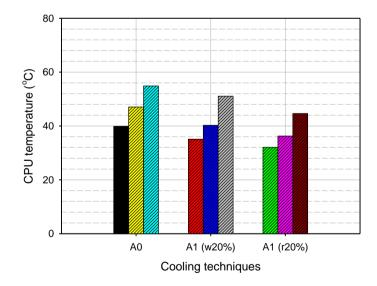
Figure 7: Comparison of CPU temperature of the vapor chamber cooling system for different cooling techniques
