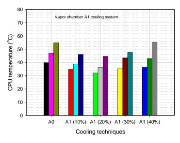
Figure 4: Variations of CPU temperature of the vapor chamber A1 cooling system for different fill ratios
