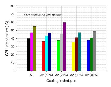
Figure 5: Variations of CPU temperature of the vapor chamber A2 cooling system for different fill ratios
