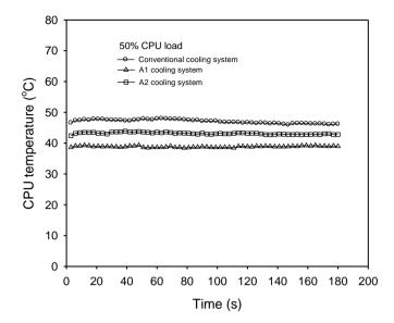
Figure 6: Variation of CPU temperature with time for different cooling techniques
