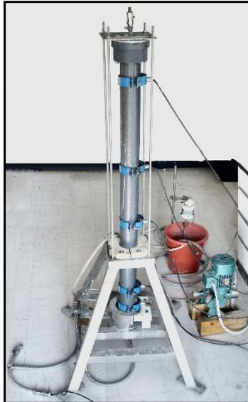
**Figure 1:** Laboratory equipment for penetrability evaluation [9-15].
