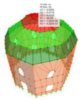
Figure 4. Location changes of the dome under the  $G+E_x$  earthquake loads of Beylerbeyi Tomb (mm)
