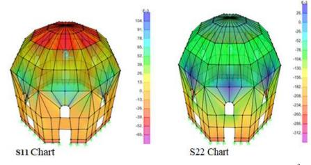
Figure 3. G loading S11 (X direction) and S22 (Y direction) tensile distribution (10<sup>-3</sup>N/mm<sup>2</sup>)
