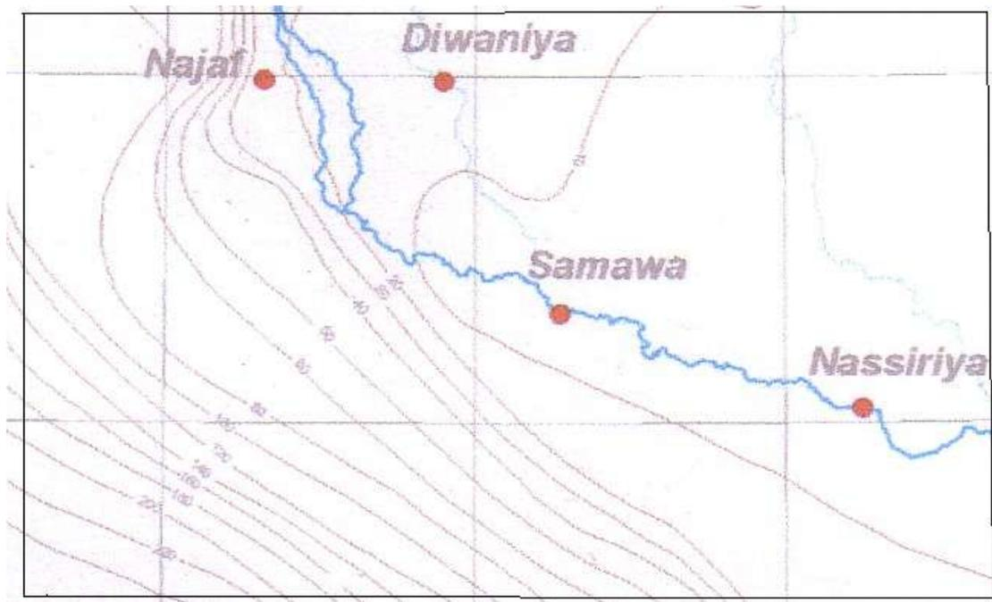
Fig.(3) : Equipotential lines of ground water (contour map ) in the study area.(Ministry of water Resources,2013).
