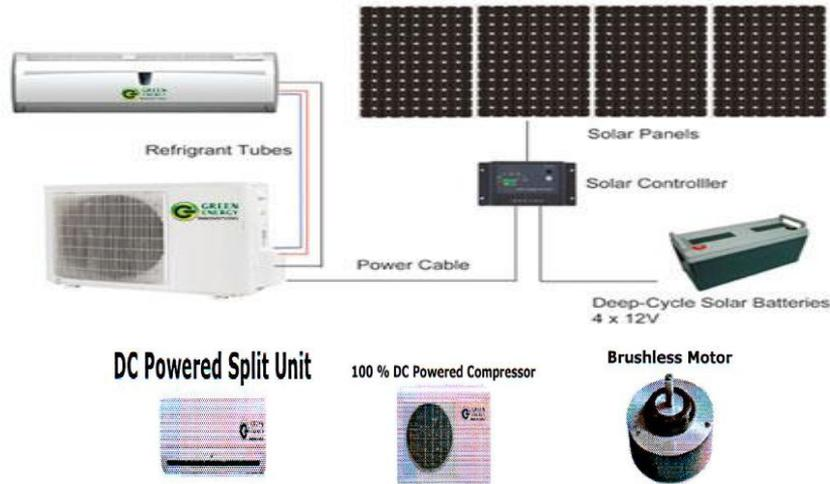
**Figure-1 : D.C. Powered Solar Air conditioner System**
