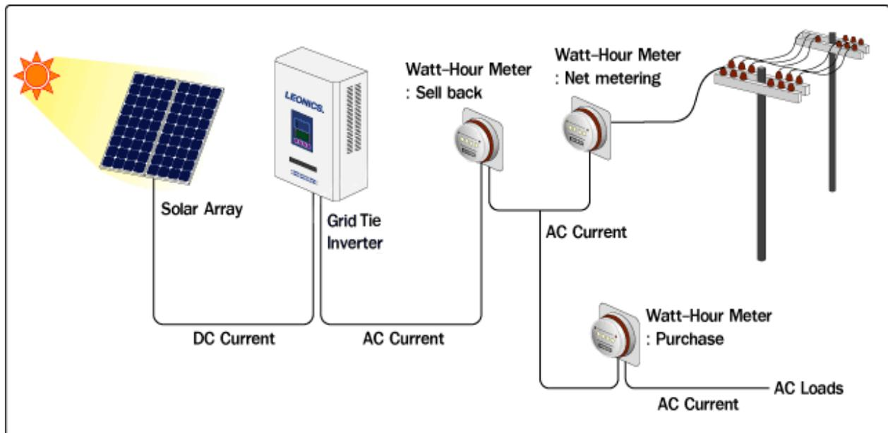
**Figure-5 : Grid Tie Solar Power System**
