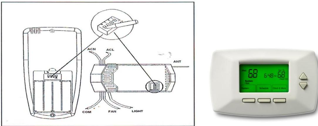
**Figure-4 : Thermostatic Ceiling Fan and Light Remote Control System**
