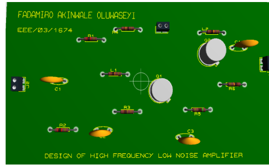
Fig 8: PCB Board layout for LNA design
