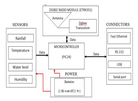
Figure 3.1 – Hardware design block diagram
