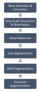
Fig. 1. Proposed System Diagram
