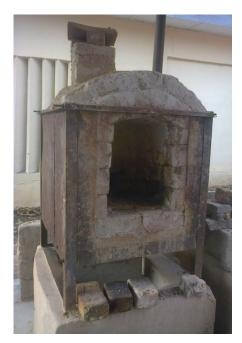
Figure 2: Prototype Design of Test Kiln Designed and fabricated by students of Industrial Department of the Federal of Technology, Akure
