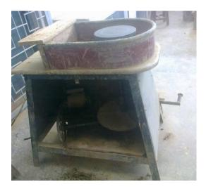
Figure: 3 Prototype Design of Electric Potters Wheel Designed and fabricated by students of Industrial Department of the Federal of Technology, Akure
