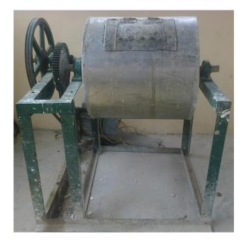
Figure 2: Prototype Design of Ball mill Designed and fabricated by students of Industrial Department of the Federal of Technology, Akure
