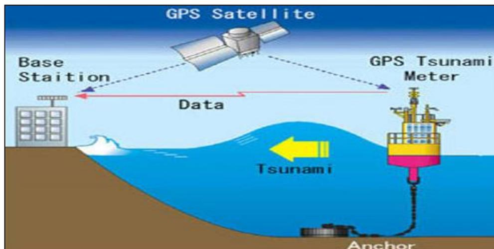
Figure 4: Tsunami Monitoring Process (source: Geogorage 2012)
