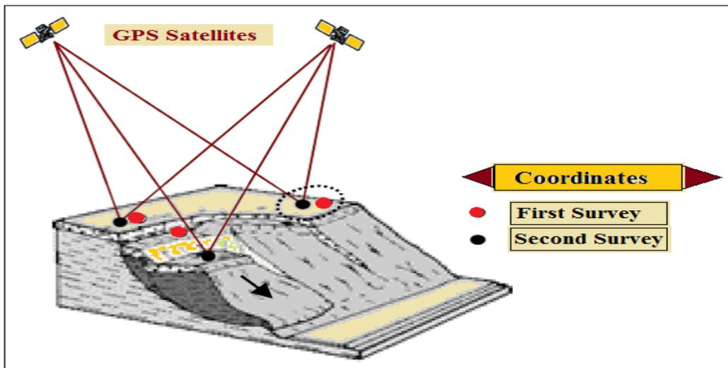
Figure 3: Landslide Monitoring Process. (Source: Abidin et al 2004)
