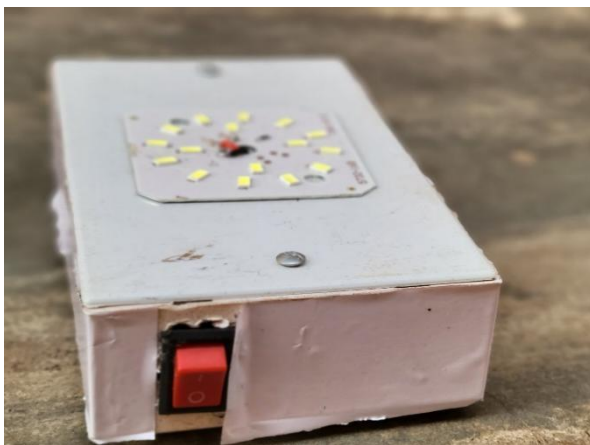
Figure 6(a). The Front view of the 5v Solar Lamp Showing the LED light and the control switch
