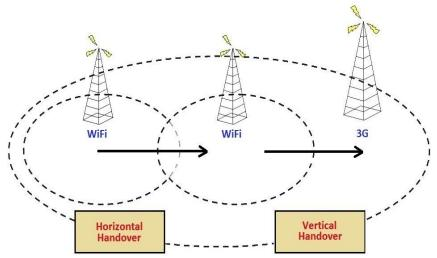
Figure 1: Graphical Illustration of Horizontal and Vertical Handovers
