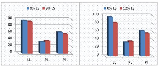
Figure 10: Atterberg Limits and Free Swell at (0%, 9%) and (0%, 12%) Lime Sludge Content
