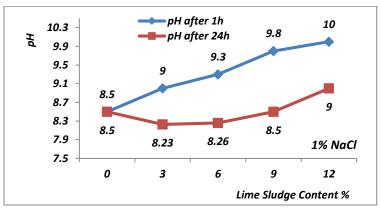
Figure 3: Variation of Soil pH By Addition of Different Ratios of (LS & 1% NaCl)
