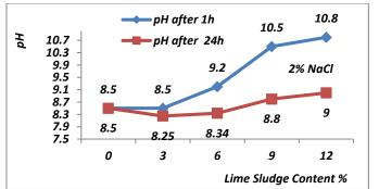
Figure 4: Variation of Soil pH by Addition of Different Ratios of (LS & 2% NaCl)
