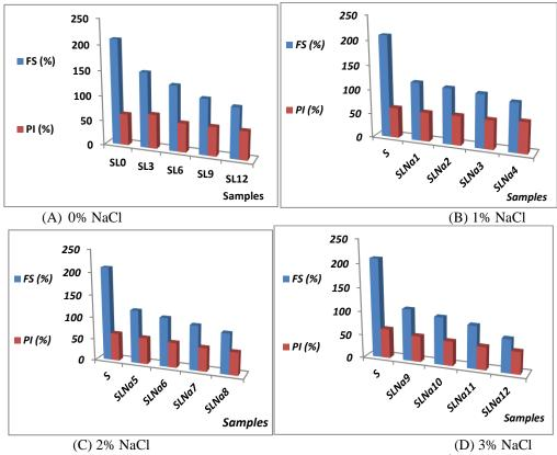
Figure 11: Effect of Additives on Plasticity Index and Free Swelling of 6<sup>th</sup> of October Soil
