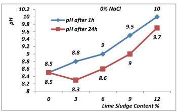
Figure 2: Variation of Soil pH by Addition of Lime Sludge in Different Ratios (3, 6, 9 & 12 %)
