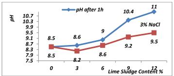
Figure 5: Variation of Soil pH by Addition of Different Ratios of (LS & 3% NaCl)
