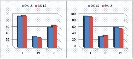
Figure 9: Atterberg Limits and Free Swell at (0%, 3%) and (0%, 6%) Lime Sludge Content
