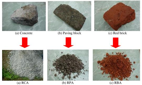
Figure 2. Process of making recycled concrete aggregate (RCA), recycled paving block aggregate (RPA), recycled brick aggregate (RBA)
