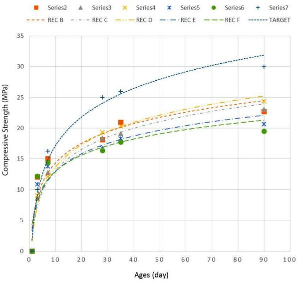
Figure 4. Comparison of timeline all recycled aggregate concrete compressive strength
