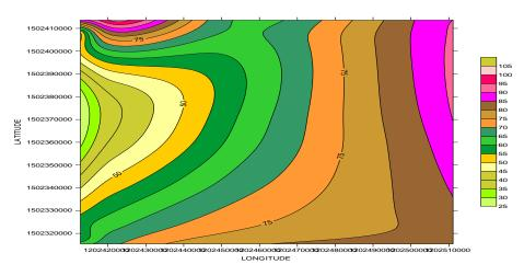
Fig.3.0: Formation temperature map within fika formation in Krumta well
