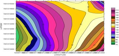
Fig.6.0: Formation temperature map within Fika formation in Wadi well
