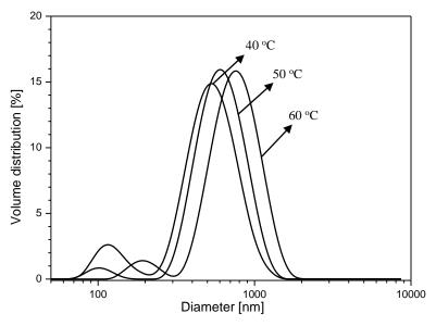
**Figure 5:** The liposomes products size distribution obtained at CO<sub>2</sub> pressure of 20 MPa with various operating temperatures.
