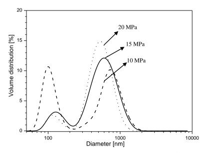
Figure 3: The liposomes products size distribution obtained at temperature of 40 °C with various CO<sub>2</sub> pressures.
