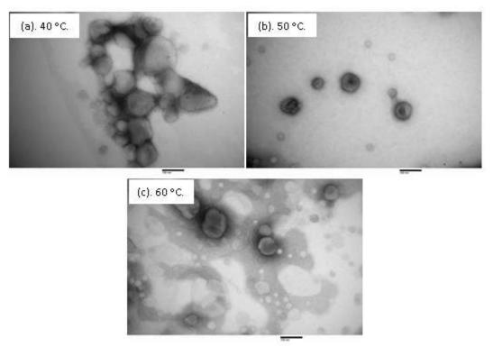
Figure 4: TEM images of liposomes products obtained at  $CO_2$  pressure of 20 MPa with various operating temperatures.
