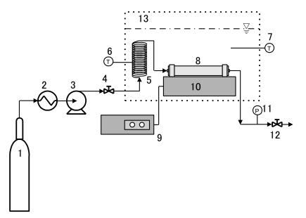
Figure 1: Experimental apparatus scheme: 1. CO<sub>2</sub> cylinder; 2. Chiller; 3. High pressure pump; 4. Needle valve; 5. SUS– 316 pre–heater; 6, 7. Temperature monitor; 8. Reactor; 9. Ultrasonic controller; 10. Ultrasonic vibrator; 11. Pressure monitor; 12. BPR; 13. Water bath.
