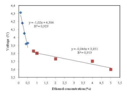
Figure 5: Relationship between voltage output of sensor vs. ethanol concentration
