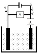
Figure 1: Electrochemical circuit of ethanol measurements
