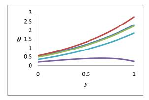
**Figure 10:** Temperature  $\theta$  versus y for Re = 1, Sc = 0.22, S = 1, m = 10, t = 1,  $\delta = 0.5$ , M = 10, Gr = 2, Gm = 1, Q = 1, F = 1 $d_1 = 0.5$ ,  $d_2 = 0.5$ , h = 1, K = 2., Pr = 0.71,1.0,1.5,2.0,2.5
