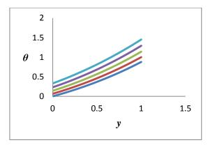
**Figure 12:** Temperature  $\theta$  versus y for Re = 1, Sc = 0.22, S = 1, Pr = 0.71, t = 1,  $\delta = 0.5$ , M = 10, Gr = 2, Gm = 1, Q = 1, F = 1m = 10,  $d_2 = 0.5$ , h = 1, K = 2., d1 = 0,0.1,0.2,0.3,0.4
