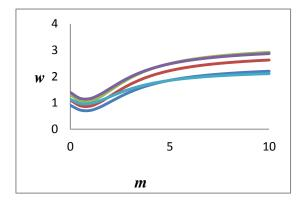
**Figure 8:** Cross Velocity w versus m for Re = 1, Sc = 0.22, S = 1, Pr = 0.71, t = 1,  $\delta = 0.5$ , M = 10, Gr = 2, Gm = 1, Q = 1, F = 1 $d_1 = 0.5$ ,  $d_2 = 0.5$ , h = 1, K = 2., y = 0,0.2,0.4,0.6,0.8
