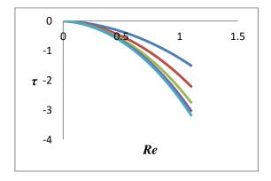
**Figure 18:** Skin friction  $\tau$  versus Re for Sc = 0.22, S = 1, Pr = 0.71, t = 1,  $\delta = 0.5$ , M = 10, Gr = 2, Gm = 1, Q = 1, F = 1,  $d_1 = 0.5$ ,  $d_2 = 0.5$ , h = 1, K = 2, m = 1,3,5,7,9 at y=1
