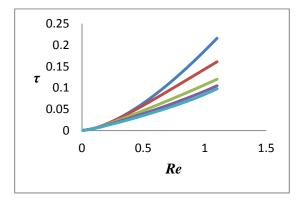
**Figure 17:** Skin friction  $\tau$  versus Re for m = 10, Sc = 0.22, S = 1, Pr = 0.71, t = 1,  $\delta = 0.5$ , M = 10, Gr = 2, Gm = 1, F = 1,  $d_1 = 0.5$ ,  $d_2 = 0.5$ , h = 1, K = 2, Q = 1, 2, 3, 4, 5 at y=0
