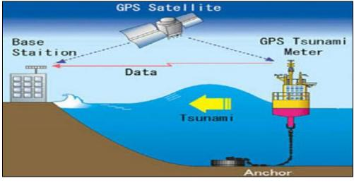
Figure 4: Tsunami Monitoring Process (
