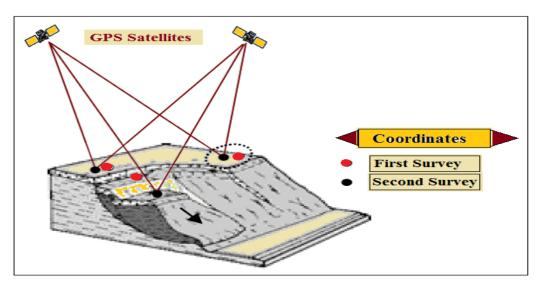
Figure 3: Landslide Monitoring Process. (Source: Abidin et al 2004)
