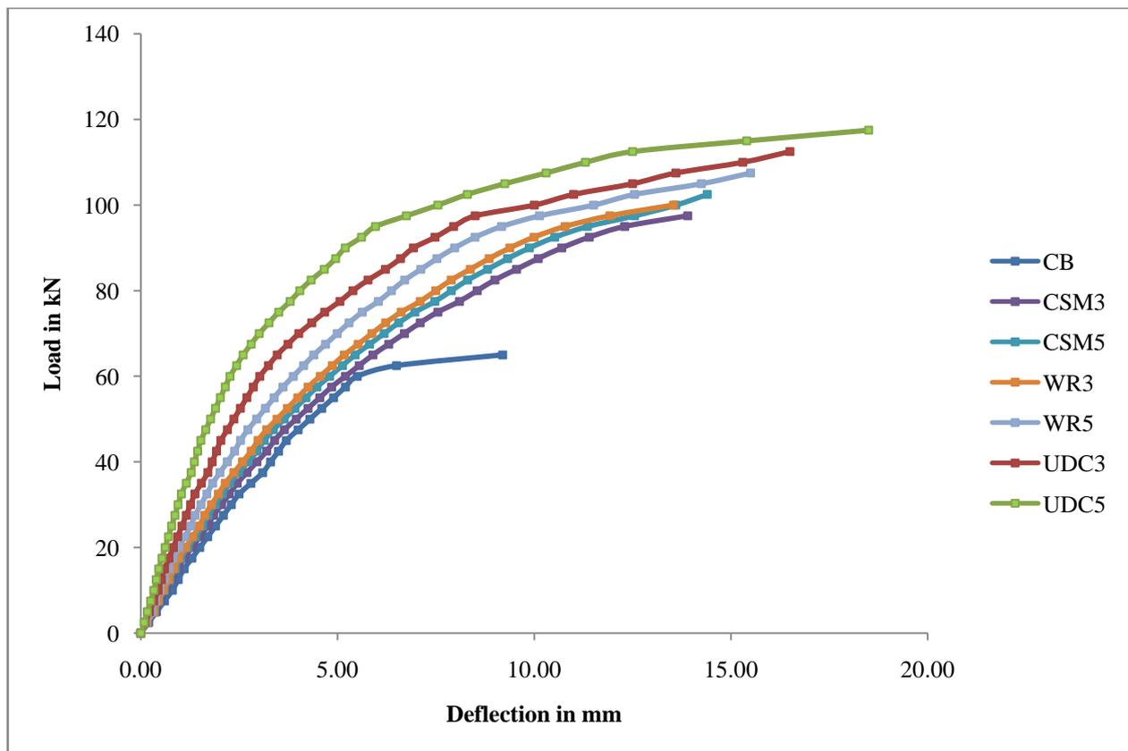
Figure 3: Load-deflection Response of Beams
