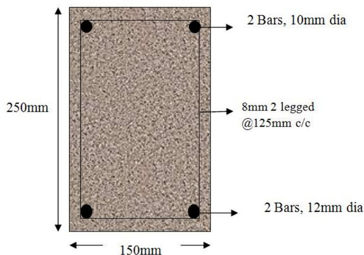
Figure 1: Reinforcement Details
