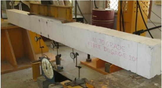
Figure .3 Test Set- Up and Instrumentation
