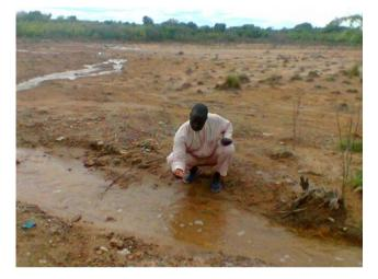
Plate 5.2 Acid Mine Drainage water at Vein 2 Baryte Mining Site The researcher is fetching water sample
