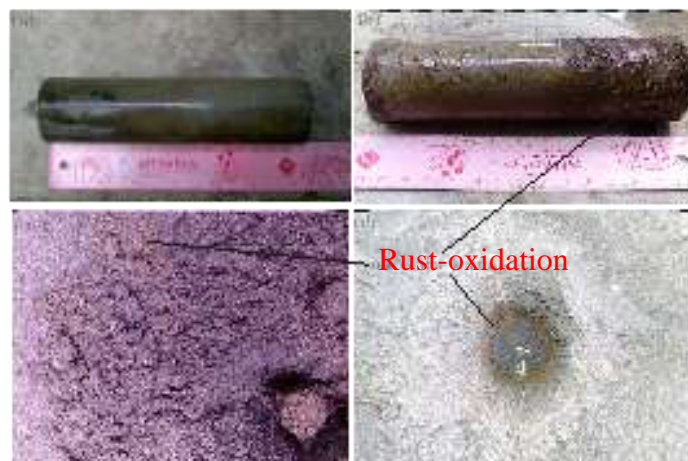
Figure 10. Metal cylinder target (a) Before observation (b) After observation, rust oxide in the bottom of the metals plate.
