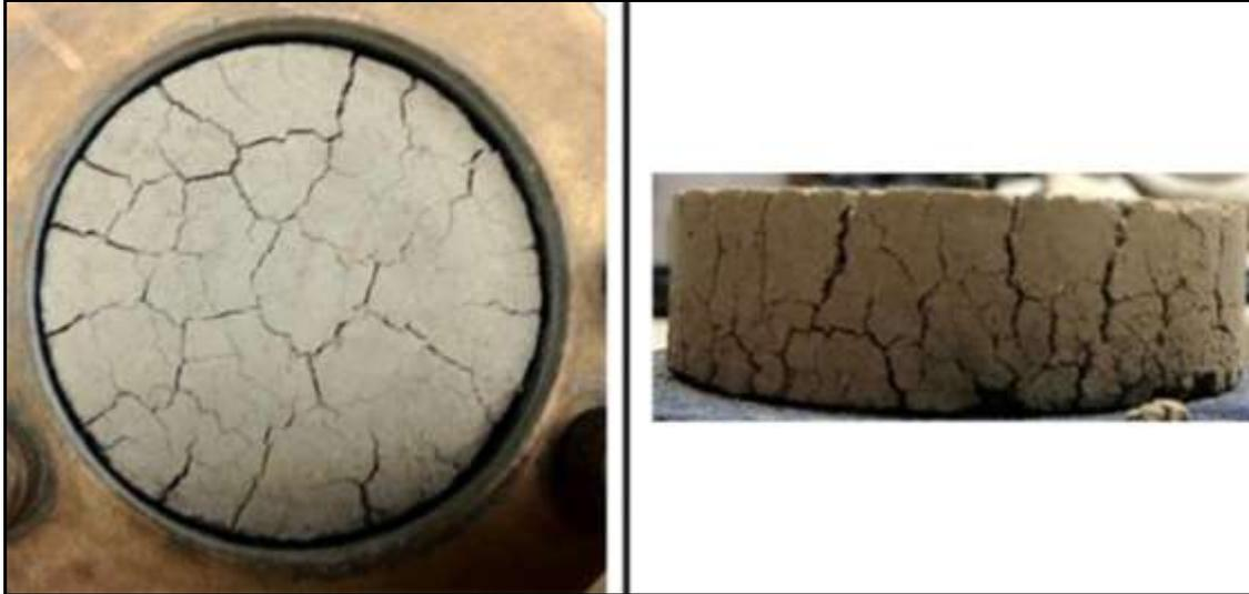
a) Top view of horizontal cracks that form on the top surface    b) Side view of the vertical cracks throughout the sample
