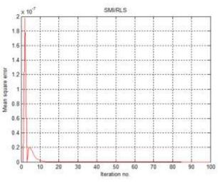
Fig. 11:Mean square error for 8 elements linear array using SMI-RLS algorithm
