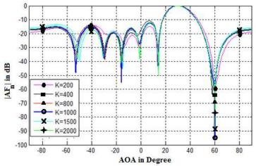
Fig. 8:Normalized array factor using SMI-LMS algorithm for  $d=0.5\lambda$
