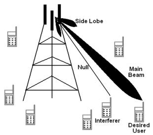
Fig. 2:Main beam toward desired user and null toward interferer
