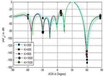
Fig. 9:Normalized array factor using SMI-RLS algorithm for  $\alpha$ =0.8 for d=0.5 $\lambda$
