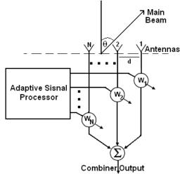
Fig. 1:Beamforming network of a smart antenna
