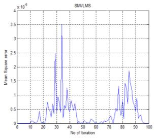
Fig. 10:Mean square error for 8 elements linear array using SMI-LMS algorithm
