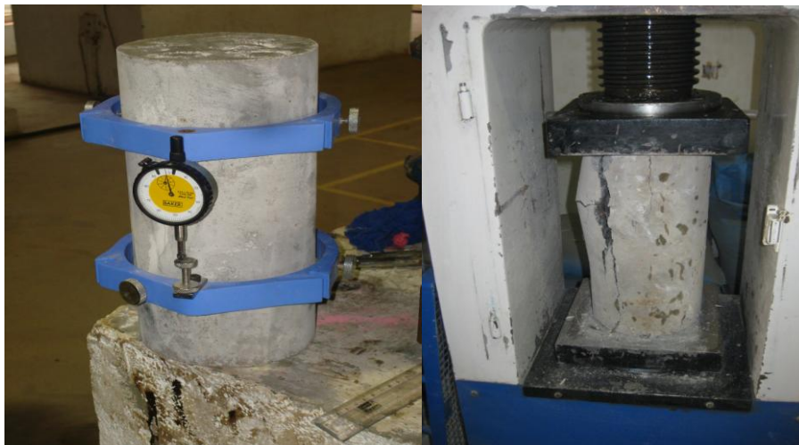
Figure 2. Compression Test of Cylinder Specimens
