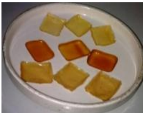
Figure 2. Crosslinked chitosan hydrogel film
