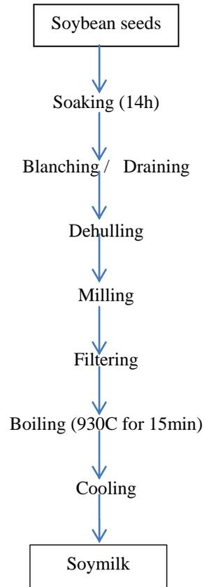
Fig.1: flow chart for soymilk (SM) production (Udeozor, 2012).
