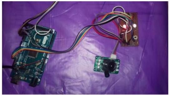
Fig 6 System in alarm mode (Red LED lights up)
