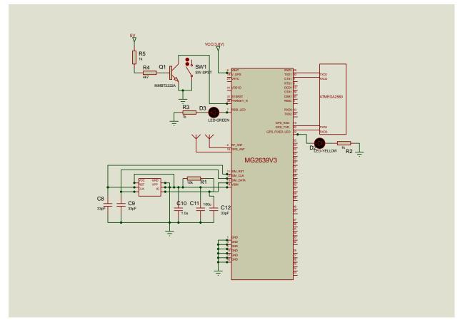
Fig. 3 MG2639 Cellular Shield
