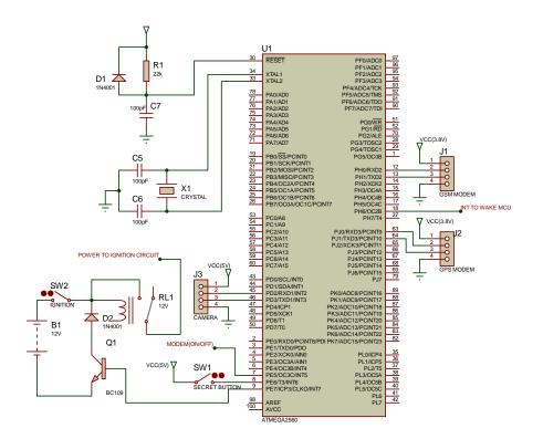
Fig 2 Atmega2560 microprocessor connections
