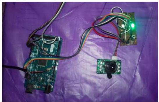
Fig 5 System in tracking mode (Green LED lights up)
