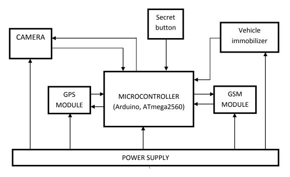
Fig 1 Block diagram of an anti-vehicle theft control system
