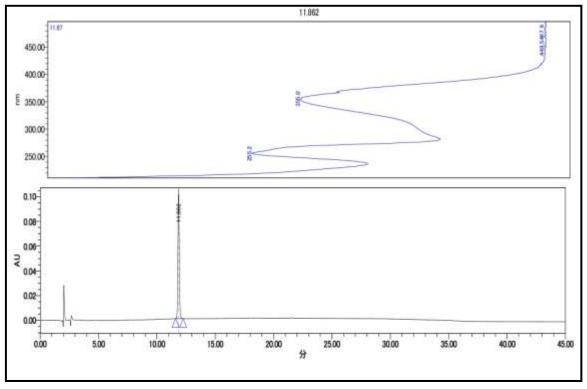
Figure 2: HPLC chromatograms and UV spectrum of antioxidant compound isolated from EtOAc\_F007 fraction of *Polyalthia longifolia* leaf at 11.862 retention time
