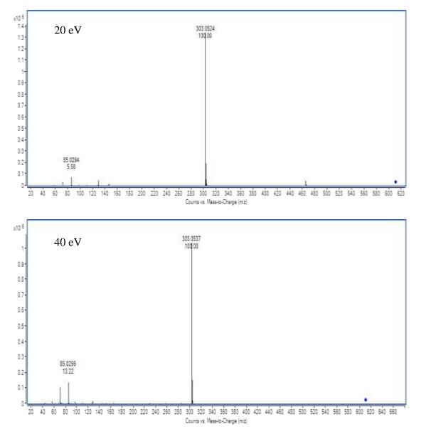
Figure 5: Typical patterns and the percentage of abundance of rutin at higher collision energy of 20 and 40 eV in ESI positive mode.
