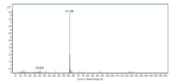
Figure 3: Positive full scan of EtOAc\_F007 isolated antioxidant compound from P. longifolia leaf using LC-QTOF-MS
