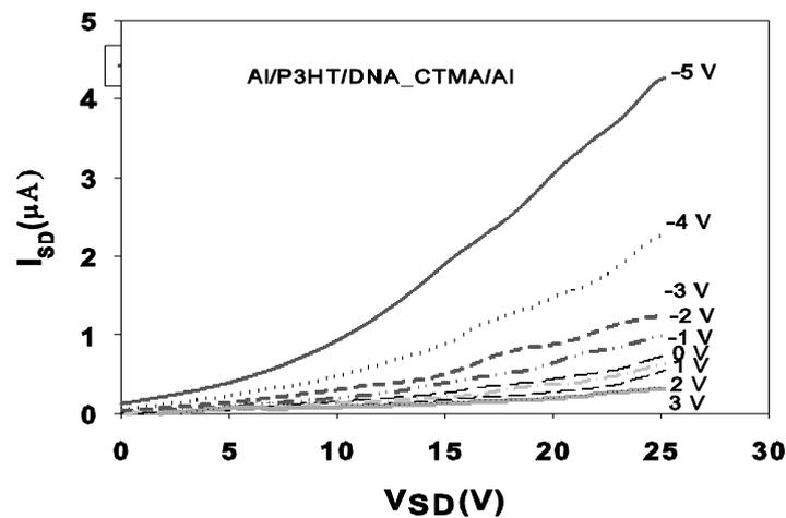
Figure 6:  $V_{SD}$  versus  $I_{SD}$  at different gate voltages.
