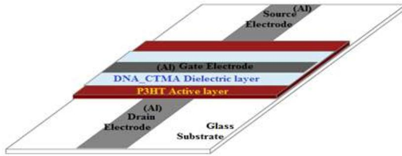
Figure 5: Fabricated device structure on glass plate
