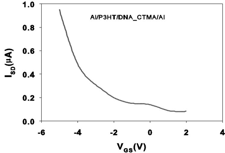
Figure 7: Transconductance curve at  $V_{SD}=10V$
