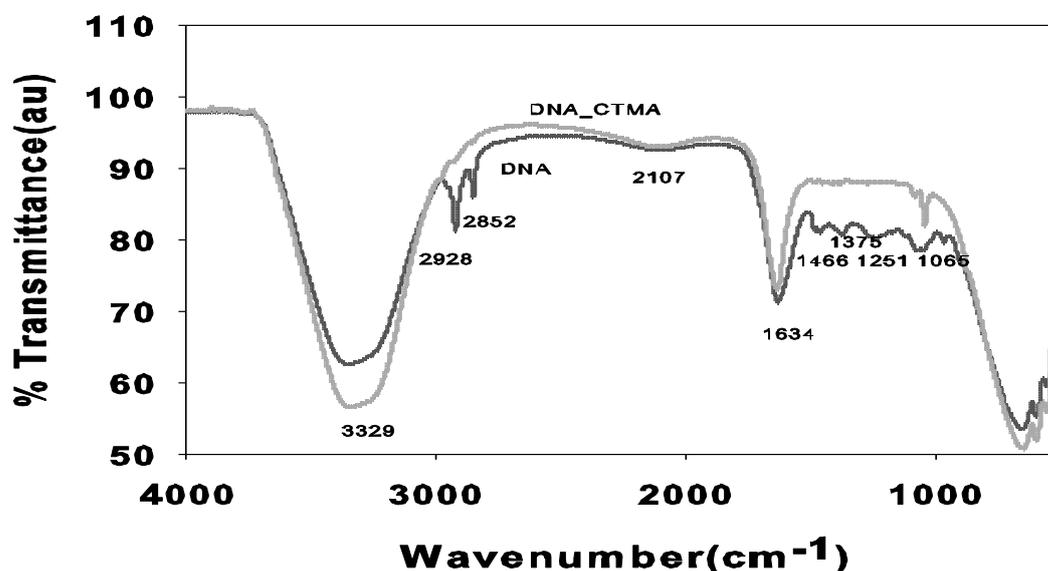
Figure 3: FTIR Spectrum of DNA and DNA\_CTMA complex.
