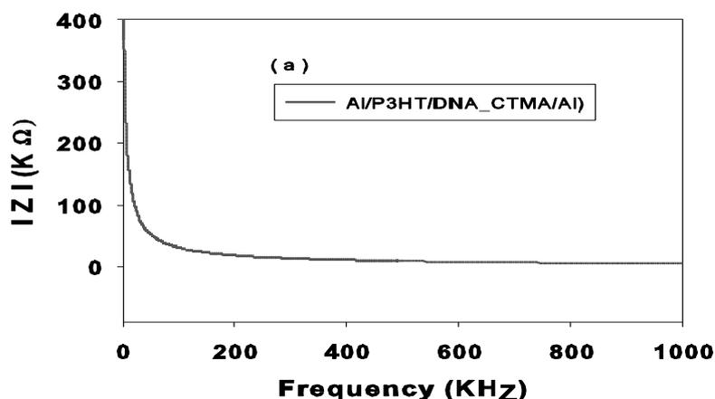
Figure 9: Device impedance versus frequency curve
