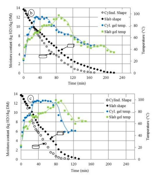
**Figure 2:** Effect of gel shape on microwave drying kinetics at different power densities: a) Ps=1 W/g; b) Ps=1.5 W/g; c) Ps=2 W/g.
