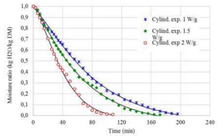
**Figure 4:** Impact of output power on drying kinetics and variation of experimental and predicted moisture ratio by Midilli model at different microwave powers (1 W/g, 1.5 W/g, 2 W/g).
