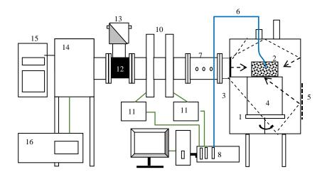
Figure 1: Schematic illustration of microwave drying with the stereo-mode cavity.
